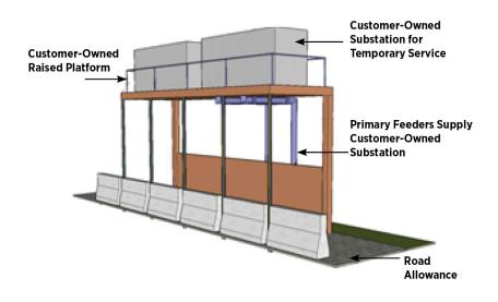
Where there's no space for temporary transformer facilities on customer property, an alternative approach may be possible whereby a temporary customer-owned substation is installed on a raised platform within the road allowance. This temporary installation is only permitted in the following circumstances:
