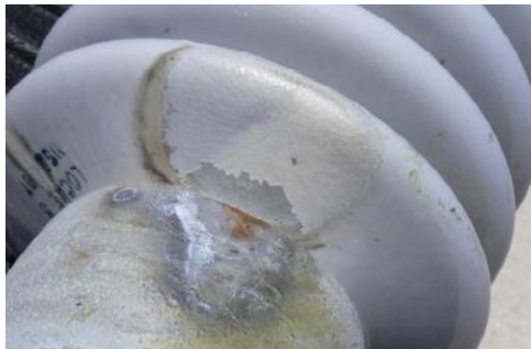
Figure 12: Close-up of Damaged Porcelain Insulator Showing Tracking
