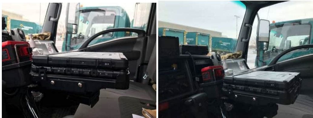
15 Figure 5: Laptop Mount Installed in Cube Van
