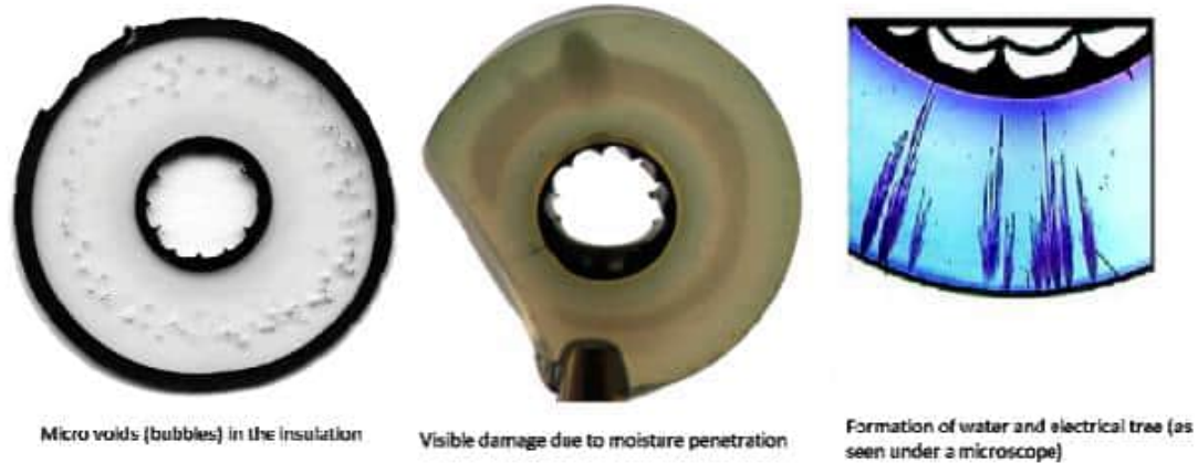
1 Figure 22: Field and Laboratory Sample of Microscopic Voids and Damage XLPE Insulation
