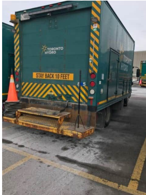
Figure 2: Corrosion on Cube Van Steps
