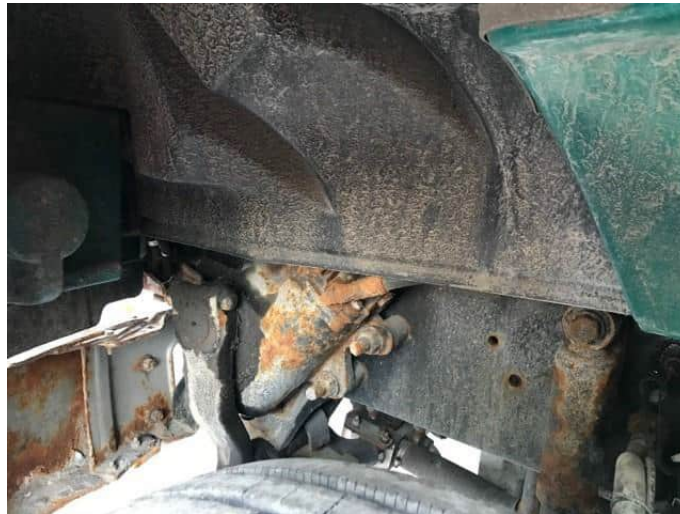
Figure 3: Axle Corrosion on Bucket Truck
