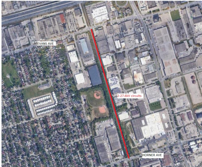
6 Figure 32: Overhead Assets in Rail Corridor
