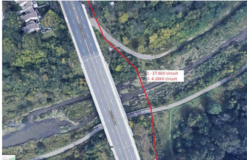
5 Figure 30: Difficult-to-Access Overhead Circuits on Humber River across Kipling Avenue
