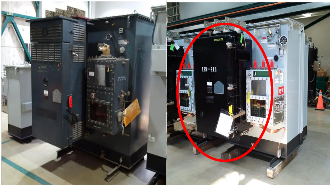
13 Figure 22: A ventilated Network Unit (Left) and a Submersible Network Unit (Right)
