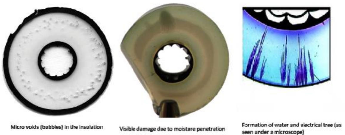
11 Figure 17: Field and Laboratory Sample of Microscopic Voids and Damage XLPE Insulation
