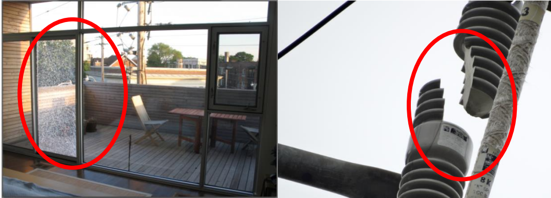
Figure 11: Porcelain Pothead Failure
