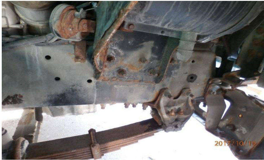
5 Figure 3: Underbody Corrosion on Bucket Truck
