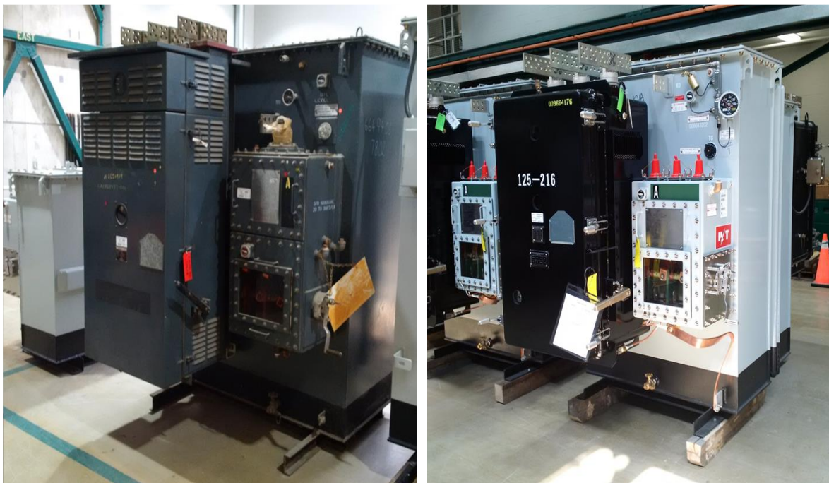
14 Figure 4: A ventilated network unit is shown on the left and a submersible network unit is shown 15 on the right. The black protector is of a submersible design, which prevents water ingress.
