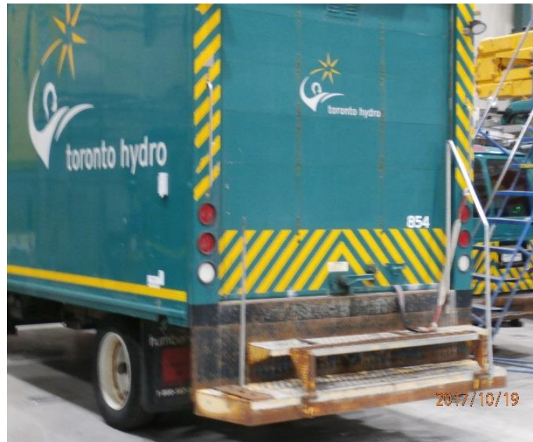
13 Figure 2: Corrosion on Cube Van Steps
